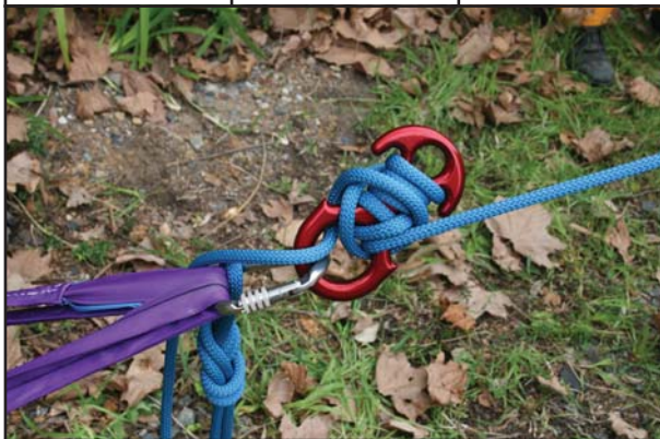
Anchor point using Tube Tape, Carabiner, Harpoon and Kermantle Rope locked off
